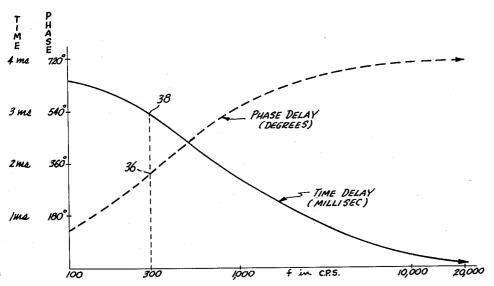
RELATIVE PHASE AND TIME DELAYS OF AUDIO SIGNAL FREQUENCY COMPONENTS
